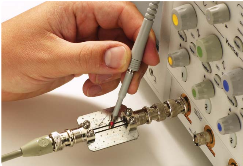
Figure 2. Fifty ohm through fixture, Agilent Technologies product number E2655-66501.
